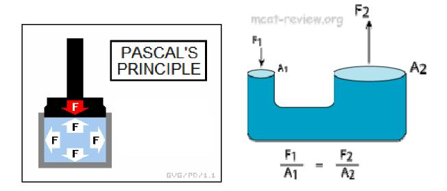
Extra credit (3 pts): For the hydraulic jack in the right diagram above, if  $F_1$  force is applied over a distance  $d_1$ , what is the displacement of the  $A_2$  area? Why does a hydraulic jack produce a mechanical advantage like a lever arm?
