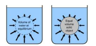
Since the "water ball" at left is exactly supported by the difference in pressure and the solid object at right experiences exactly the same pressure environment, it follows that the buoyant force on the solid object is equal to the weight of the water displaced (Archimedes' principle) BECAUSE the water ball is in static equilibrium where the water ball weight (downward force) is balanced by the upward buoyancy force so that  $F_{net} = 0$ , hence there is not acceleration of the water ball.
