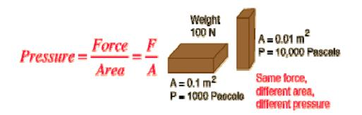
**Pascal's Principle or Law.** Pressure is transmitted undiminished in an enclosed static fluid. A force applied to one section of an enclosed liquid at rest will be transferred to the entire liquid with the same amount of force. This is why a hydraulic jack works and you can blow out the bottom of a bottle by pushing on its top.
